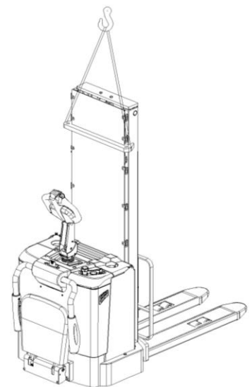
Fig.5: Lifting with a crane
