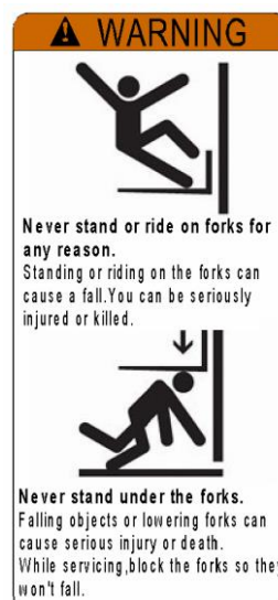
Sign not under, on forks (N)
